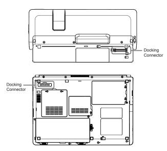
The images above show the notebook and the docking station. Please take note of the placement of the docking ports. When the notebook is placed the right way up, the docking connectors will be on the same side. Ensure that these are aligned correctly before trying to dock the notebook to the docking station.
